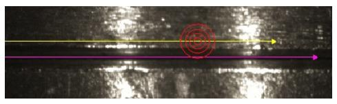
In the second photo, the system automatically aligns the laser path with the weld seam. The red welding target is now properly placed on the seam. The result is an approved part each time.
